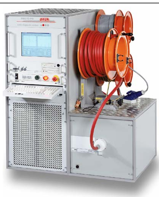
Figure 9: VLF Test And Diagnosis (DF&PD) System 57 kV rms , 80 kV DC up to 20 \mu F
