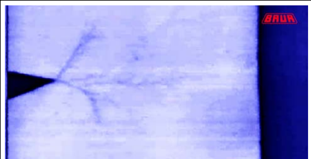
Figure 7: Electrical Treeing On a Cable Sample (Section of a XLPE Cable) With a Defect (Needle Electrode Inside Insulation) at VLF Voltage (0.1 Hz Frequency)
