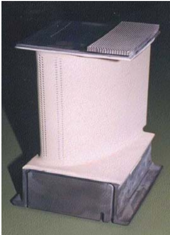
Figure 4: Vane Segment - TBC Coating Done By LPPS Plasma Spray
